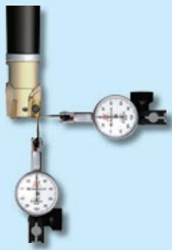
Test radial runout and axial runout with 2 measuring devices.
